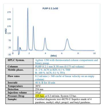
With more than double the back pressure at similar linear flow rates of 340 cm/hr. PLRP-S cannot be supported by process instruments whereas the Simulated-Monolith<sup>TM</sup> can. With 4,000 to 6,000 angstroms through pores these monoliths are stable and unlike soft gel or any other stationary phase on the market, they do not leach and therefore contaminate the purified products.
