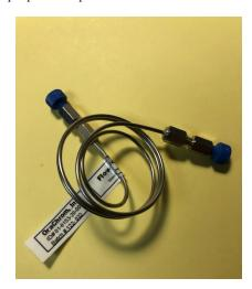
Coiled column of 1 mm ID x 50 cm length Simulated-Monolith<sup>TM</sup> STYROS® Polymeric.
