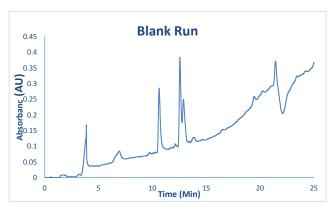
Should this blank run be deducted from the previous chromatogram, a chromatogram with flat baseline results that is consistent with full digestion of the protein.
