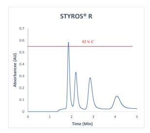
The retention times have shifted similarly without affecting the ratios of the peaks or their relative intensities. What is again clear is the increased hydrophobicity of the polymeric media and its increased retentivity of it.
