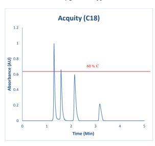
Considering the retention times as well as the peak ratio it is sate to consider the trapping as being complete.
