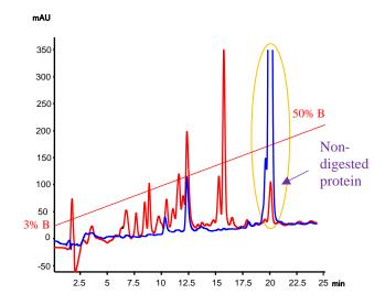
The chromatogram shows the digestion to be over 95 % complete,
