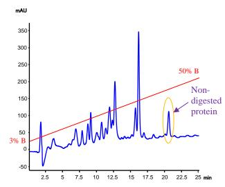
The enzyme column (StyrosZyme® TPCK-Trypsin) is a 2.1x100 mm Narrow Bore column followed by a 2.1x100 mm reversed phase (STYROS® 1R), also Narrow Bore reversed phase column to trap and map the resulting digested peptides.
