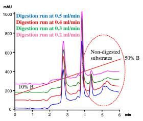
The digestion increases as the linear velocity decreases from 900 cm/hr. to 400 cm/hr. based on an empty column of 2.1mm ID.
