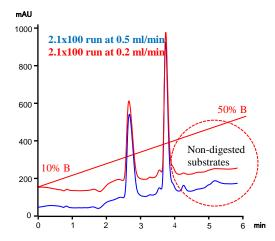
It is reasonable to conclude that the full digestion of Oxidized B-Chain at a set temperature of  $37^{\circ}$ C and at a pH 8.5 using 0.1 M Tris buffer depends on both the length of the column used and the linear velocity of the digestion.
