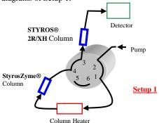
In the second position, the enzyme column is removed from the line and only the reversed phase STYROS® 2R column remains.
