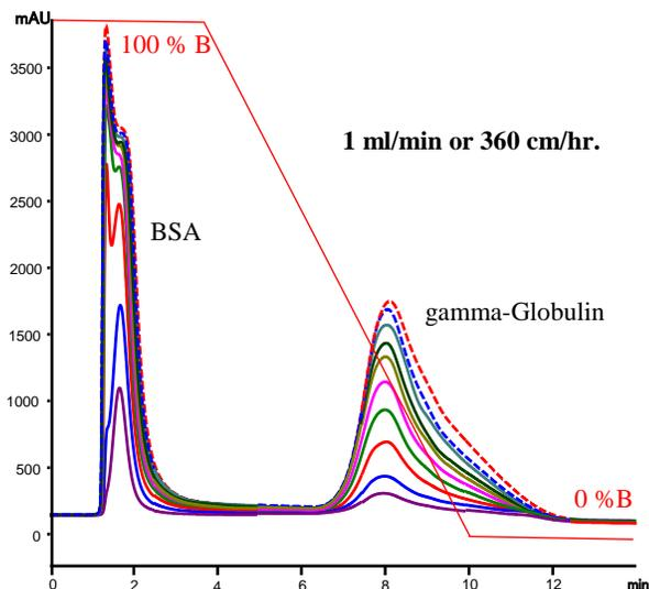
The column is run at volumetric flow rates of 1 and 2 ml/min. The linear velocities are 360 and 720 cm/hr. respectively.
