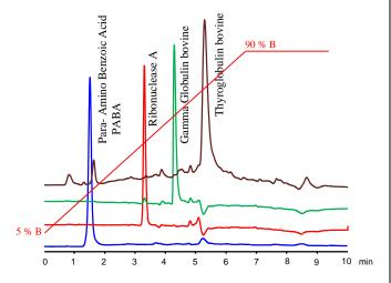
A STYROS® 2R narrow bore column of 2.1 mm ID was used for the separation to minimize the use of sample and the generation of waste as well as to increase sensitivity.
